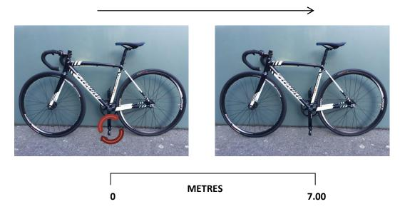
Pedal starts in vertical at 0 and rotates in direction of red arrow above and must be back within 7.00m (or whichever your roll out gearing restriction is). Gearing is either under or over, there is no such thing as close/grey area.
